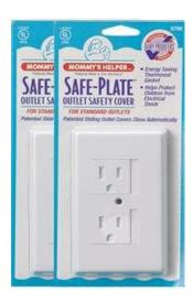
These devices are not expensive and can be retrofitted into older homes. They employ a spring-loaded shutter mechanism that only allows electricity to flow when equal pressure is applied simultaneously to both shutters (for example, when an electrical plug is inserted). During unused conditions, both shutters are closed and openings are covered.
